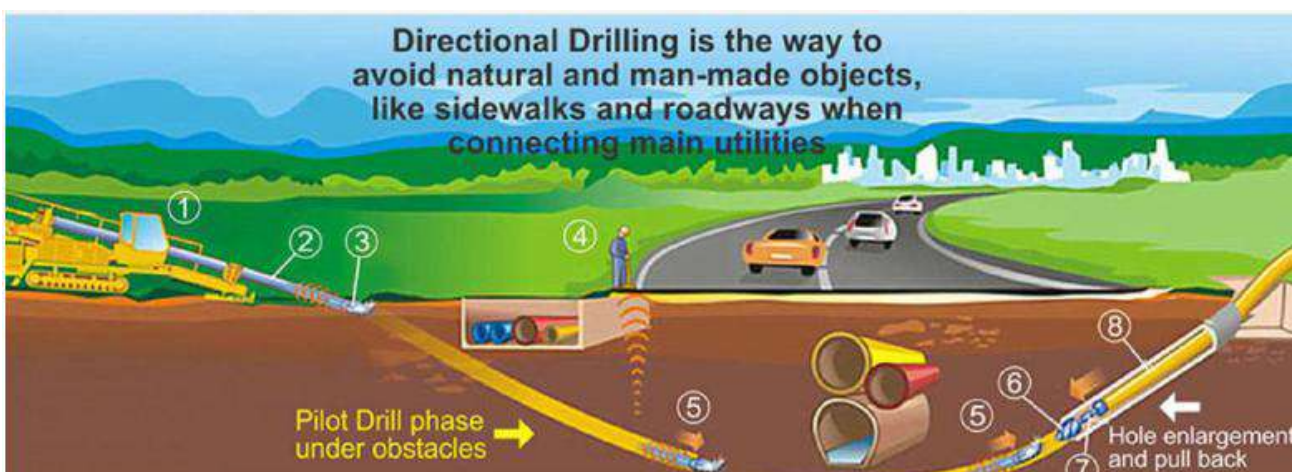
FIGURE 1.18 TYPICAL HORIZONTAL DIRECTIONAL DRILLING (HDD) PROCESS
